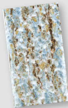
Post-galvanized 85 µm after 12 weeks
