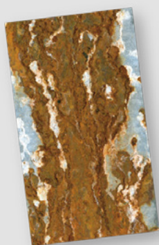
Galvanized 20 µm after 6 weeks
